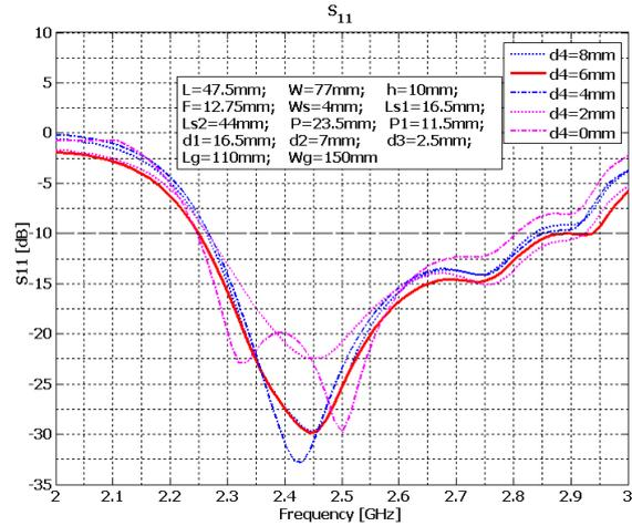
Fig. 6. Simulated return loss  $S_{11}$  at different values of  $d_4$  while other parameters are fixed.
