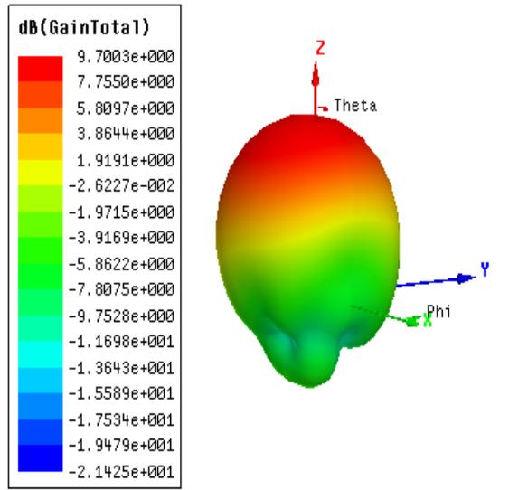
Fig. 7. Simulated (a) 2-D and (b) 3-D radiation patterns of the proposed antenna at 2.44 GHz.
