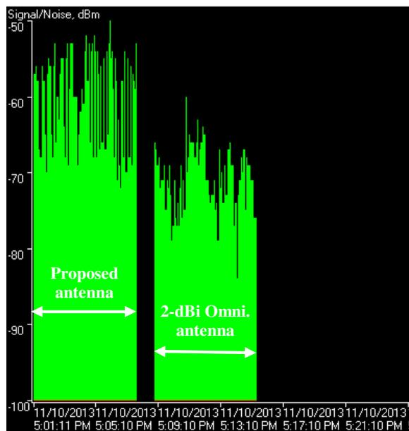
Fig. 14. Compared antenna gains under non-line-of-sight condition.
