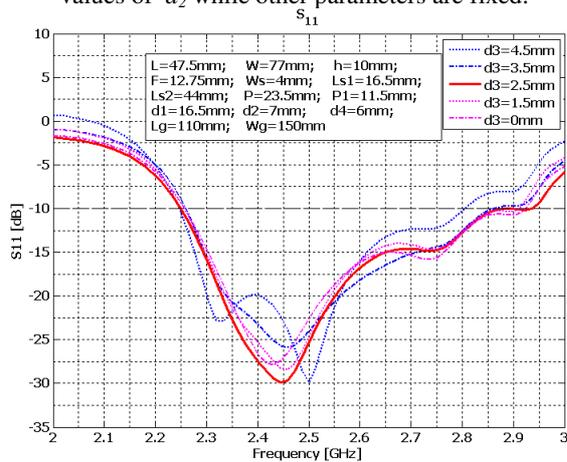
Fig. 5. Simulated return loss  $S_{11}$  at different values of  $d_3$  while other parameters are fixed.
