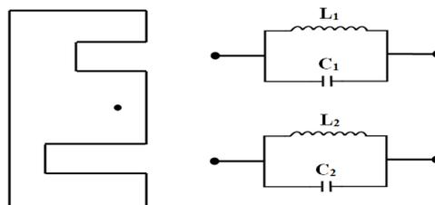
Fig. 2. Resonance mechanism of the E-shaped patch antenna.
