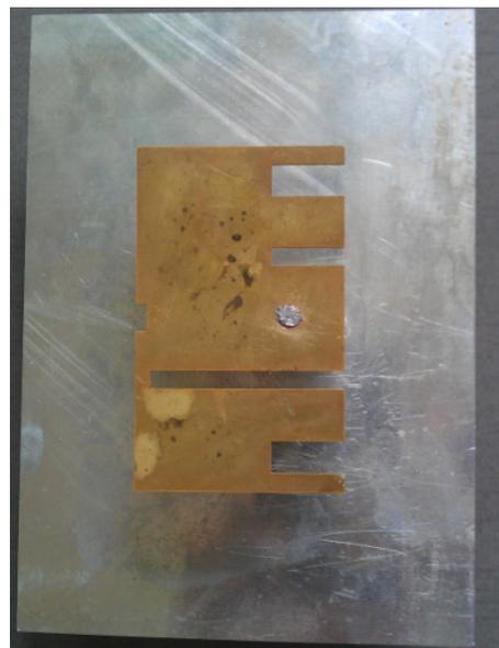
Fig. 12. Front view of the prototype of the proposed E-shaped patch antenna.
