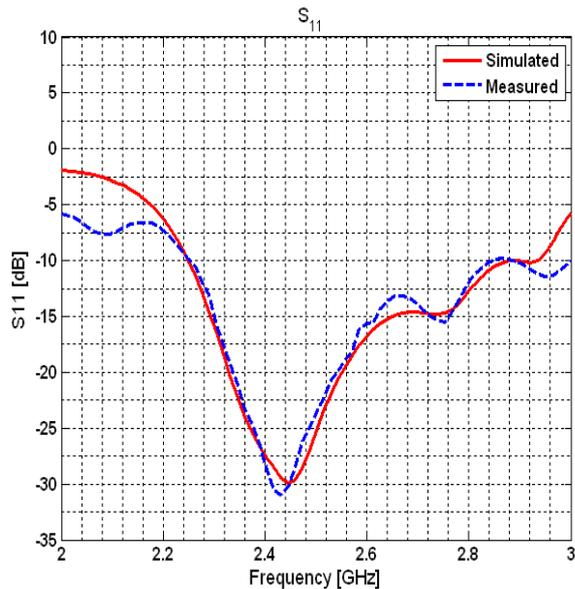
Fig. 13. Measured and simulated return loss  $S_{11}$  of the proposed antenna.
