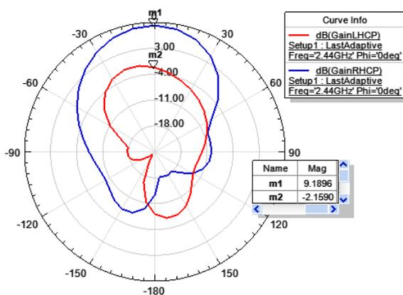
Fig. 10. The radiation patterns of left-hand circular polarization (red) and right-hand circular polarization (blue) in the  $xz$  plane.
