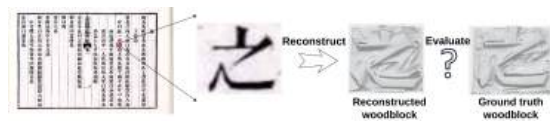
Figure 2. The evaluation problem: How to measure the quality of the generated character woodblock with the ground-truth one?
