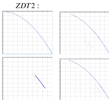
Fig. 6. Visualization of the interactive method on ZDT2 in orders: (1 st : Without interactive, 2 nd : Rays Replacement, 3 rd : Rays Redistribution, 4 th : Value Added Niching).
