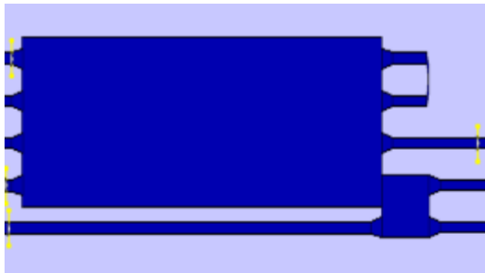
Figure 4. Photonic circuit for implementing the 4-point Haar transform using 4x4 MMI cascaded with a 2x2 MMI coupler.
