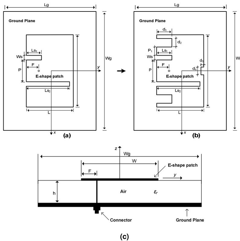
Fig. 1. Geometry and dimensions of the E-shaped patch antenna: (a) the conventional form, (b) the proposed antenna, and (c) side view of the antenna.
