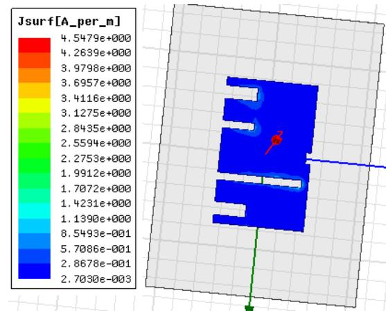
Fig. 11. Current distribution on the patch of the proposed antenna.
