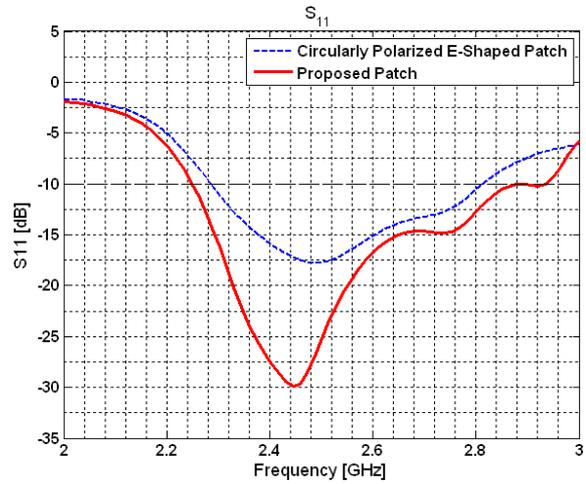
Fig. 8. Comparison of return loss  $S_{11}$  between the conventional E-shaped patch antenna (dash line) and the proposed antenna (solid line).
