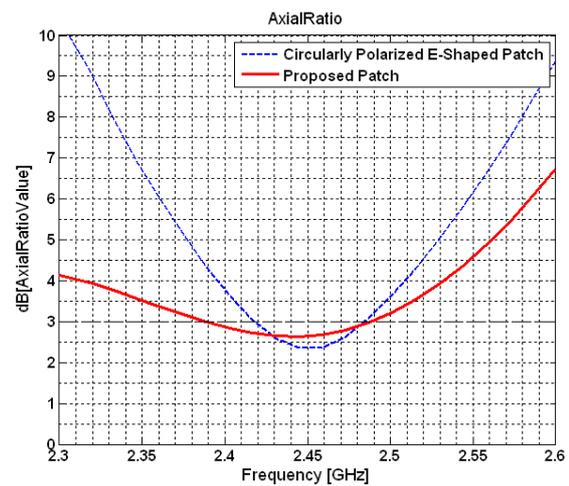
Fig. 9. Comparison of axial ratio between the conventional E-shaped patch antenna (dash line) and the proposed antenna (solid line).
