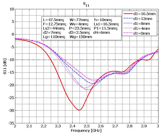
Fig. 3. Simulated results of return loss  $S_{11}$  at different values of  $d_1$  while other parameters are fixed.
