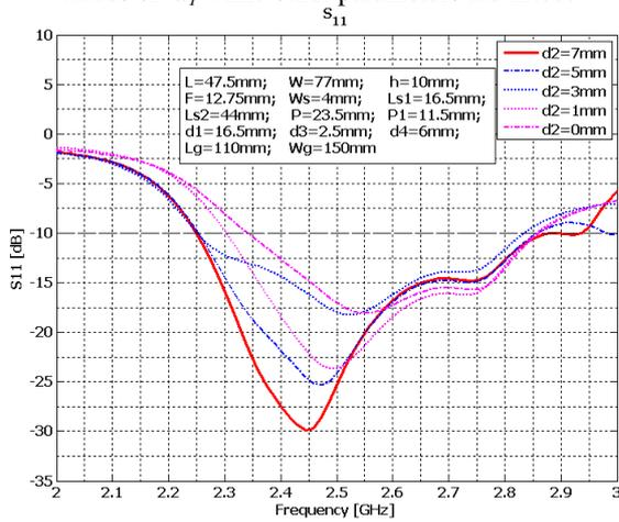
Fig. 4. Simulated results of return loss  $S_{11}$  at different values of  $d_2$  while other parameters are fixed.
