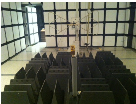
Fig. 7: Antenna measurement using a vector network analyzer in an anechoic chamber
